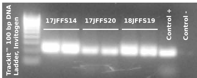
Figure 5.8. Agarose gel electrophoresis internal PCR products of Agaz1 microsatellite amplification from JFFS faecal samples.
